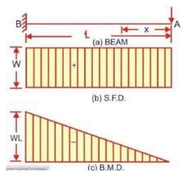
At section x from the end A, Fx = -W1 and is constant for any position of the section. The S.F.D. will, therefore, be rectangle of height W. Bending moment at a section x from end A is given by:
