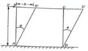
Fig. 2.3 : Strain Energy Stored Due to Shear Stress
