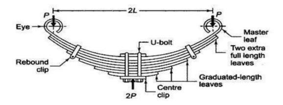
When no external load is acting, the spring is curved or cambered. Camber is the perpendicular distance between the reference line and the master leaf and its magnitude is such that the spring is approximately straight under the max static load. Center of the spring is fixed to the axle of the automobile.
