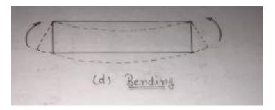
• **Bending Loads**: The loads which tend to cause a certain degree of curvature or bending in the member is called bending loads.
