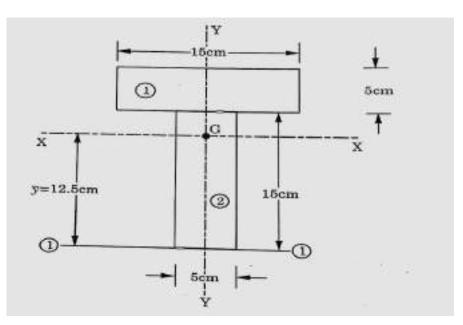
Solution. Let us split this T-section into two components- Component (1) and component (2) As this section is symmetrical about YY-axis, therefore, the centroid will lie on this axis.
