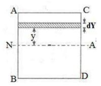
Let us assume one strip of thickness dy and area dA at a distance y from the neutral axis as displayed in above figure. Let us determine the force acting on the layer due to bending stress and we will have following equation
