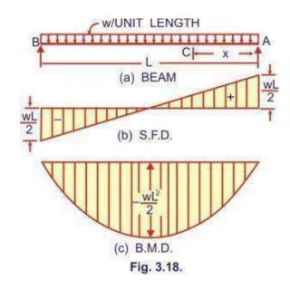
The reaction  $R_A = R_B = \frac{wL}{2}$  (due to symmetry)
