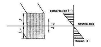
Figure Bending Stress Distribution in a Beam
